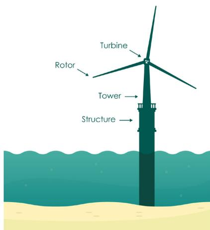
Fig. 2: Main parts of an offshore wind turbine. (Source: ABS Group)
