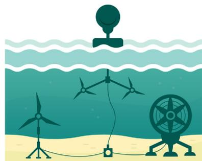
Fig. 1: Wave (top) and Tidal (bottom) Energy Technology (Source: Marine Renewables Canada)
